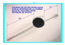
Stress cracks revealed by the inside bore, under the oil port hole.
